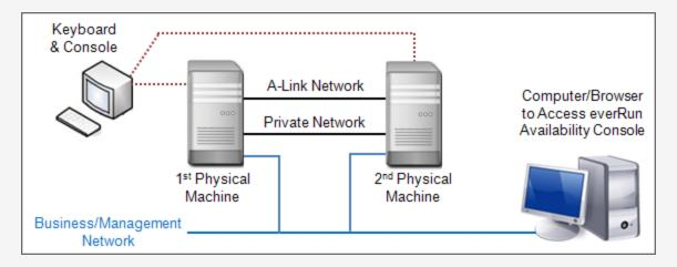
Note: When installing software on the first PM, connect the keyboard and monitor to the first PM.
