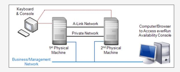
**Note**: When installing software on the first PM, connect the keyboard and monitor to the first PM. When installing software on the second PM, connect the keyboard and monitor to the second PM. When software installation is complete, disconnect the keyboard and monitor from the system.
